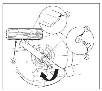
Figure 7. Tightening the Mower Blade for Installation
